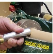
For the novices amongst us **NEVER** use Roughing Gauge on faceplate work, i.e. bowl turning, the shaft of the chisel is not strong enough to cope with the lateral forces applied.
