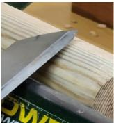
Then, using a much smaller  $\frac{1}{2}$ " skew, Roger showed how to master cutting small bevels and radii. The smaller skew had the edges of the chisel shaft ground to a soft radius to make for easier movement on the tool rest.
